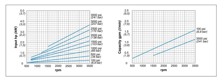
Note: These curves depict maximum working pressures. Pressures shown in order code are full-flow relief set pressures. 175 SUS Hydraulic Oil @ 120° F (49° C)
