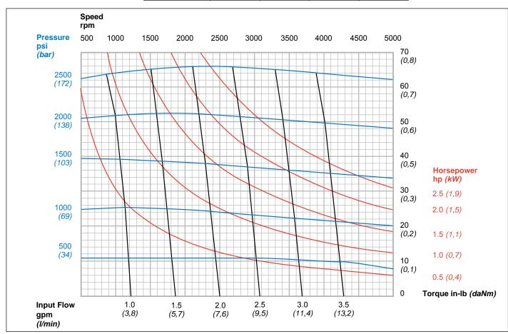
Note: These curves depict maximum working pressures. Pressures shown in order code are full-flow relief set pressures. 175 SUS Hydraulic Oil @  $120^{\circ}$  F ( $49^{\circ}$  C)
