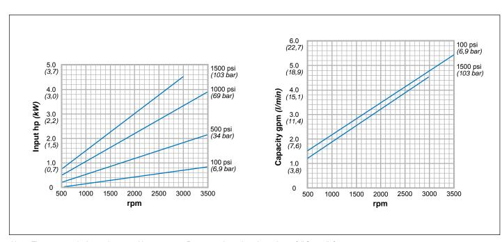
Note: These curves depict maximum working pressures. Pressures shown in order code are full-flow relief set pressures. 175 SUS Hydraulic Oil @  $120^{\circ}$  F ( $49^{\circ}$  C)
