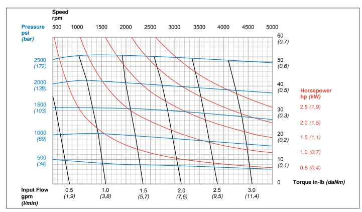
Note: These curves depict maximum working pressures. Pressures shown in order code are full-flow relief set pressures. 175 SUS Hydraulic Oil @ 120° F (49° C)
