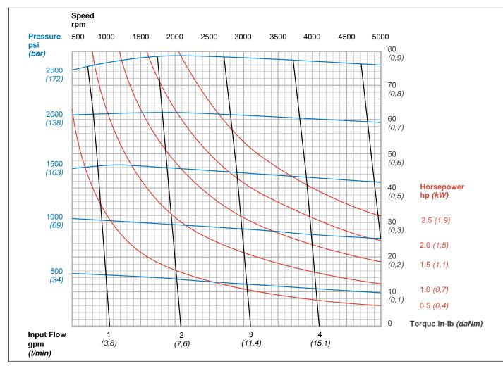
Note: These curves depict maximum working pressures. Pressures shown in order code are full-flow relief set pressures. 175 SUS Hydraulic Oil @ 120° F (49° C)
