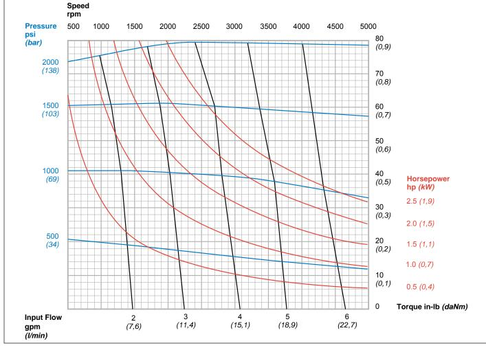
Note: These curves depict maximum working pressures. Pressures shown in order code are full-flow relief set pressures. 175 SUS Hydraulic Oil @ 120° F (49° C)
