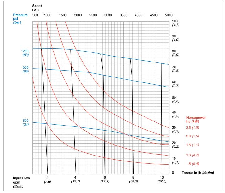
Note: These curves depict maximum working pressures. Pressures shown in order code are full-flow relief set pressures. 175 SUS Hydraulic Oil @  $120^{\circ}$  F ( $49^{\circ}$  C)
