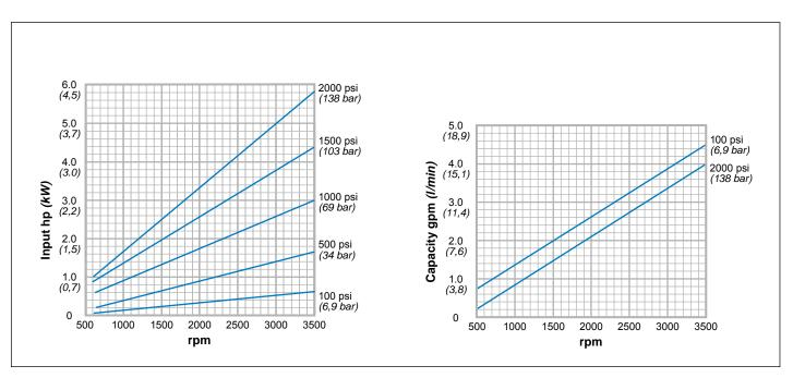
Note: These curves depict maximum working pressures. Pressures shown in order code are full-flow relief set pressures. 175 SUS Hydraulic Oil @ 120° F (49° C)
