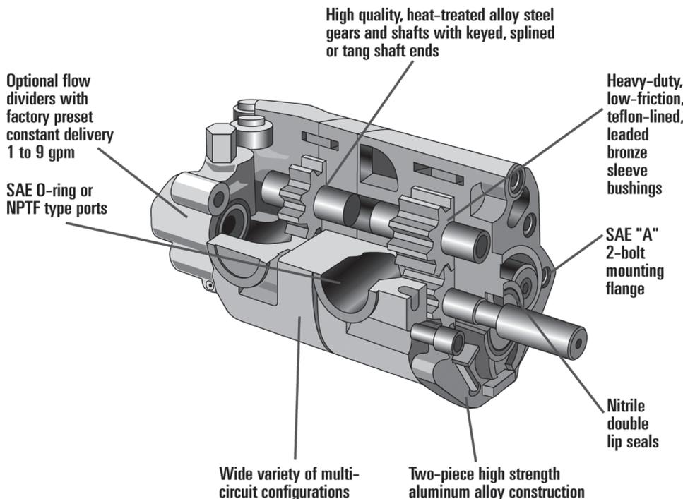
The Webster line is comprised of the B, YB and YC (shown here) series of hydraulic gear pumps and motors.
