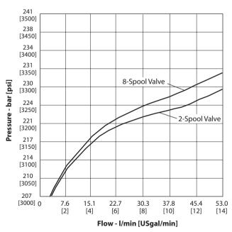
With work port relief SVLP set to 206 bar [3000 psi] at 2.8 l/min [0.75 US gal/min]
