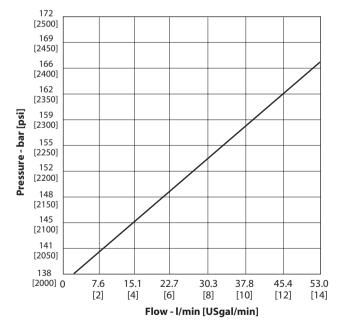
With system relief SVPR set to 138 bar [2000 psi] at 2.8 l/min [0.75 US gal/min]
