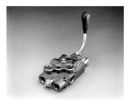
Single spool directional control valve with parallel circuitry. 38 l/min [10 US gal/min] maximum flow. 207 bar [3000 psi] maximum pressure.
