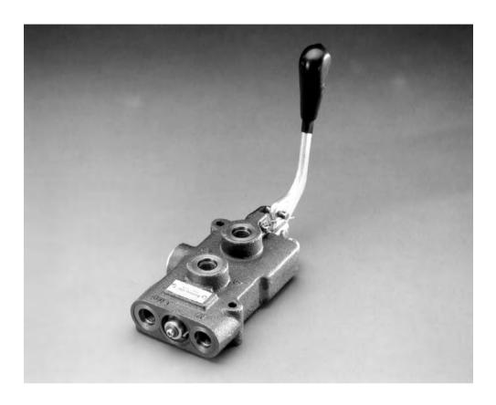
Single spool monoblock valve. 26.4 l/min [7 US gal/min] maximum flow. 138 bar [2000 psi] maximum pressure with relief. 207 bar [3000 psi] maximum pressure without relief.
